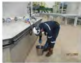
3. Connect bonding (sampling and blanket)
